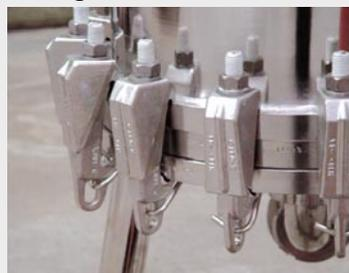
Closing mechanism with swing bolts.
